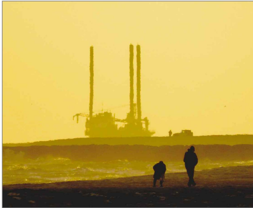
A self-elevating barge off Smith Point conducts seafloor survey work for the Sunrise Wind farm in 2020.
